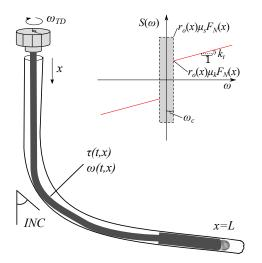
Fig. 1. Schematic indicating the distributed drill string of length L lying in deviate borehole. Inset: Schematic illustrating the friction source term  $S(\omega, x)$ . The shaded region represents the angular velocities for which a constant value of static torque is assumed and the red curve indicates the dynamic torque as a function of angular velocity.
