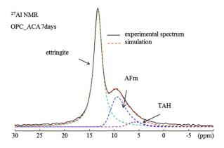
**Fig. 12.** <sup>27</sup>Al MAS NMR spectra (9.4 T,  $\nu_R$  = 20 kHz) of 7 days hydrated paste OPC–ACA in the Al(VI) sixfold range. A simulation is presented where the dotted line in red is the simulation of the experimental spectrum and the dotted lines the fitted model of ettringite (Lorentz model, δ = 13.3 ppm), AFm (Czjzek model, δ = 10.0 ppm, C<sub>Q</sub> = 1.3 MHz) and the third aluminate hydrate (TAH) [66] (Czjzek model, δ = 6.5 ppm, C<sub>Q</sub> = 3.3 MHz).
