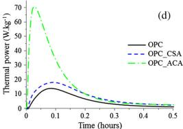
**Fig. 1.** Cumulative heat of OPC, OPC\_CSA and OPC\_ACA pastes (a) and heat flow development, as a function of time, between 0–160 h (b), 0 and 8 h (c), and 0–0.5 h (d).
