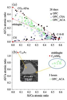
**Fig. 7.** Al/Ca atomic ratio plotted against Si/Ca atomic ratio for individual X-ray microanalyses of the matrix of cement pastes at 28 days (a) and the hydrated shell in the OPC\_ACA after 3 h (b). Red points represent pure phases and red lines, a mix between two pure phases.
