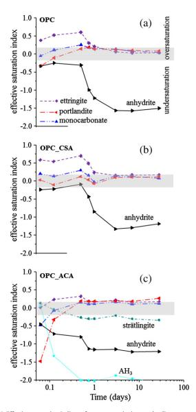
**Fig. 14.** Effective saturation indices of gypsum, ettringite, portlandite monocarbonate and AH<sub>3</sub>, strätlingite (in the case of OPC\_ACA) of hydrated pastes OPC (a), OPC\_CSA (b) and OPC\_ACA (c) as a function of time. The shadowed area indicates saturation.
