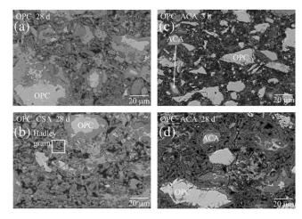
**Fig. 6.** Backscattered electron images of hydrated OPC (a), OPC\_CSA (b) and OPC\_ACA (d) pastes hydrated at 28 days and the OPC\_ACA paste hydrated at 3 h (c). The formation of separated hydration shells (Hadley grains) is clearly visible in OPC\_CSA (b). At 3 h, in the OPC\_ACA (c), ACA reacts (small particle already fully reacted) and ettringite needles can be seen.
