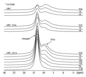
**Fig. 11.**  $^{27}$ Al MAS NMR spectra (9.4 T,  $\nu_R$  = 20 kHz) of hydrated pastes OPC, OPC\_CSA, OPC\_ACA in the Al(VI) sixfold frequency range.
