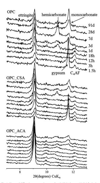
Fig. 4. Observed diffraction patterns between 7 and 13° 20 degrees (CuK $_{\alpha}$ ) for hydrated OPC, OPC\_CSA and OPC\_ACA pastes.
