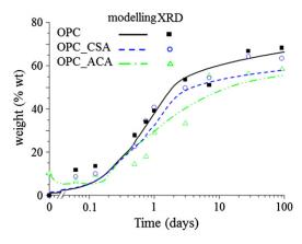
**Fig. 17.** Amount of X-ray amorphous and AFm hydrated products deduced by XRD/Rietveld analysis as a function of hydration time. Lines refer to the results of thermodynamic modeling.
