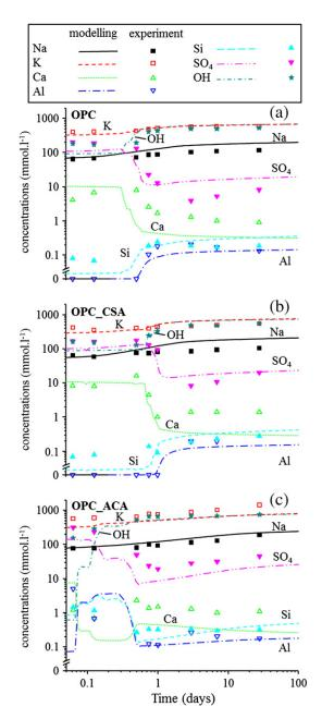
**Fig. 13.** Modeled concentrations in the liquid phase (lines) compared to the experimentally determined concentrations (symbols) of hydrated pastes OPC (a), OPC\_CSA (b) and OPC\_ACA (c) as a function of time.
