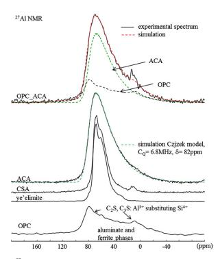
**Fig. 9.** <sup>27</sup>Al MAS NMR spectra (9.4 T,  $\nu_R$  = 20 kHz) of anhydrous materials OPC, CSA, ACA and the anhydrous blend OPC\_ACA. The NMR spectrum of synthetic ye'elimite is presented for comparison with CSA spectrum. The green dotted line represents the simulation of the experimental spectrum ACA using the Czjzek model.
