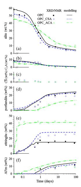
**Fig. 3.** Amounts of alite (a),  $C_3A$  (b), anhydrite (c), portlandite (d), ettringite (e) deduced by XRD–Rietveld analysis and AFm (f) deduced by  $^{27}Al$  NMR (CO<sub>3</sub>–AFm is assumed) as a function of time. Lines in (a and b) are calculating using the cement hydration model of Parrott and Killoh [73], and lines in (b, d, e, and f) refer to the results of thermodynamic modeling.
