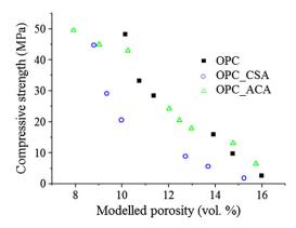
Fig. 19. Relation between compressive strength and modeled porosity.
