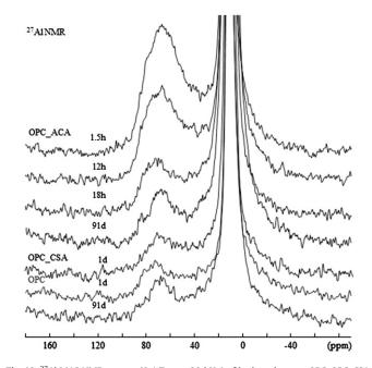
**Fig. 10.** <sup>27</sup>Al MAS NMR spectra (9.4 T,  $\nu_R$  = 20 kHz) of hydrated pastes OPC, OPC\_CSA, OPC\_ACA in the Al(IV) fourfold frequency range.
