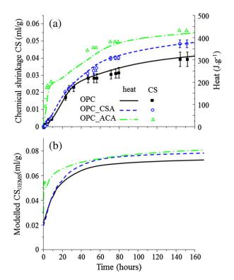
**Fig. 2.** Calculated chemical shrinkage CS relative to the blended cement content (symbol) compared with cumulative heat (line), as a function of time (a). Modeled chemical shrinkage as a function of time calculated by GEMS (b).
