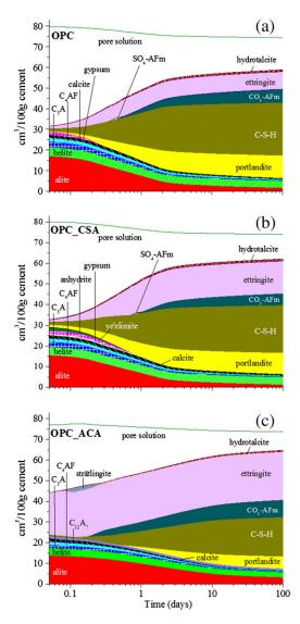
**Fig. 16.** Modeled changes during the hydration of OPC (a), OPC\_CSA (b) and OPC\_ACA (c) as a function of time. Volume expressed as  ${\rm cm}^3/100~{\rm g}$  unhydrated blended cement.
