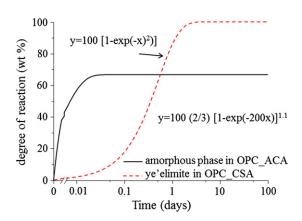
**Fig. 15.** Degree of reaction of ye'elimite (dotted line) and amorphous phase  $C_{12}A_7$  in OPC\_ACA (plain line) as a function of time used as input in the thermodynamic model.
