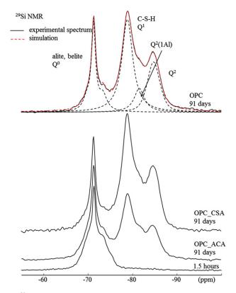
**Fig. 8.** <sup>29</sup>Si MAS NMR spectra (9.4 T,  $\nu_R$ =4.5 kHz) of OPC, OPC\_CSA hydrated at 91 days and OPC\_ACA pastes hydrated at 1.5 h and 91 days. The dotted line in red is the simulation of the experimental spectrum OPC.
