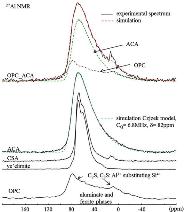
**Fig. 9.**  $^{27}\text{Al}$  MAS NMR spectra (9.4 T,  $\nu_R = 20$  kHz) of anhydrous materials OPC, CSA, ACA and the anhydrous blend OPC\_ACA. The NMR spectrum of synthetic ye'elimite is presented for comparison with CSA spectrum. The green dotted line represents the simulation of the experimental spectrum ACA using the Czjzek model.
