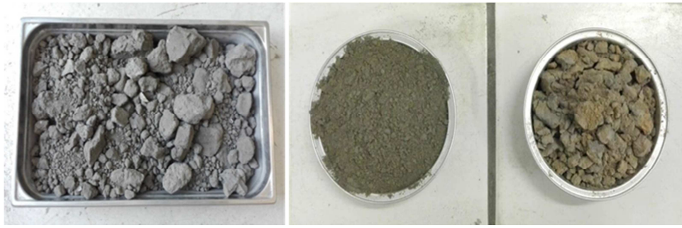
Fig. 2. Process of treatment (from left to right: sediment after drying, after grinding, after thermal treatment)
