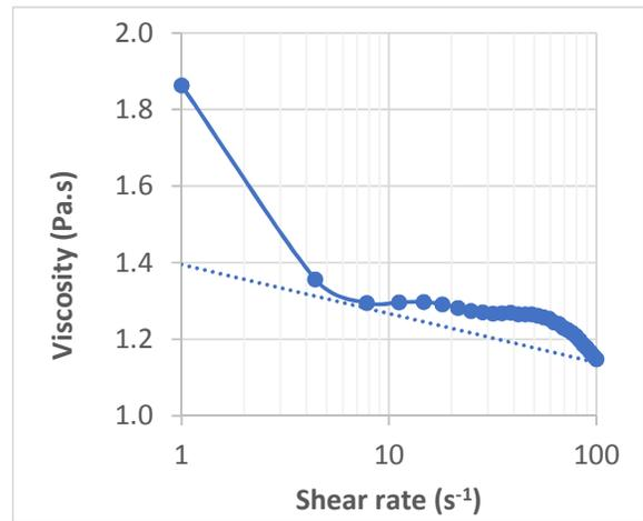
Fig. 11. The data from the 2<sup>nd</sup> mix fitted perfectly the Bingham model
