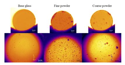
**Fig. 7.** IR image (up) and zoomed IR images (down) of base glass and sintered sample obtained with different grain size powders.
