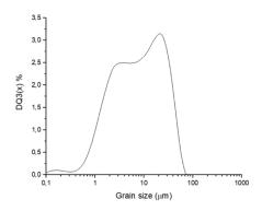
**Fig. 4.** Measured grain size after 88 h of milling.
