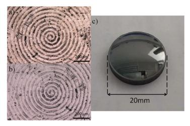
**Fig. 8.** Pictures taken by optical microscopy of aluminum block (a), resulting footprint from the aluminum block on TGS lens (b) and full lens after molding (c).
