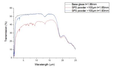
**Fig. 6.** Transmission spectra of the base glass synthesized by melt-quenching and of samples obtained by SPS sintering of powder  $<100 \, \mu m$  and powder  $>100 \, \mu m$ .
