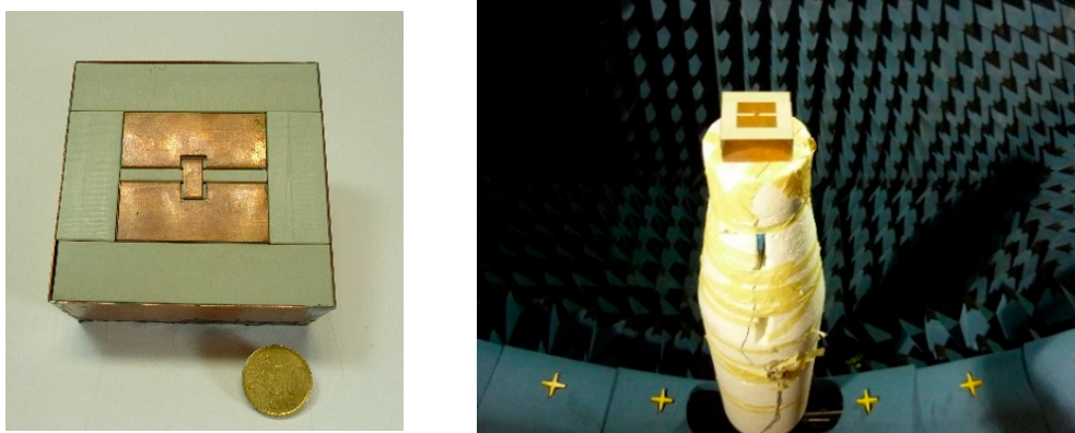
Figure 10. Photograph of the manufactured antenna (left) and radiating measurements (right).
