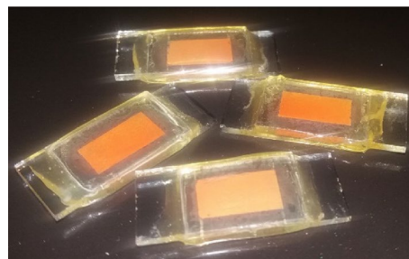
Fig. 2 Assembled bixin-sensitized solar cell
