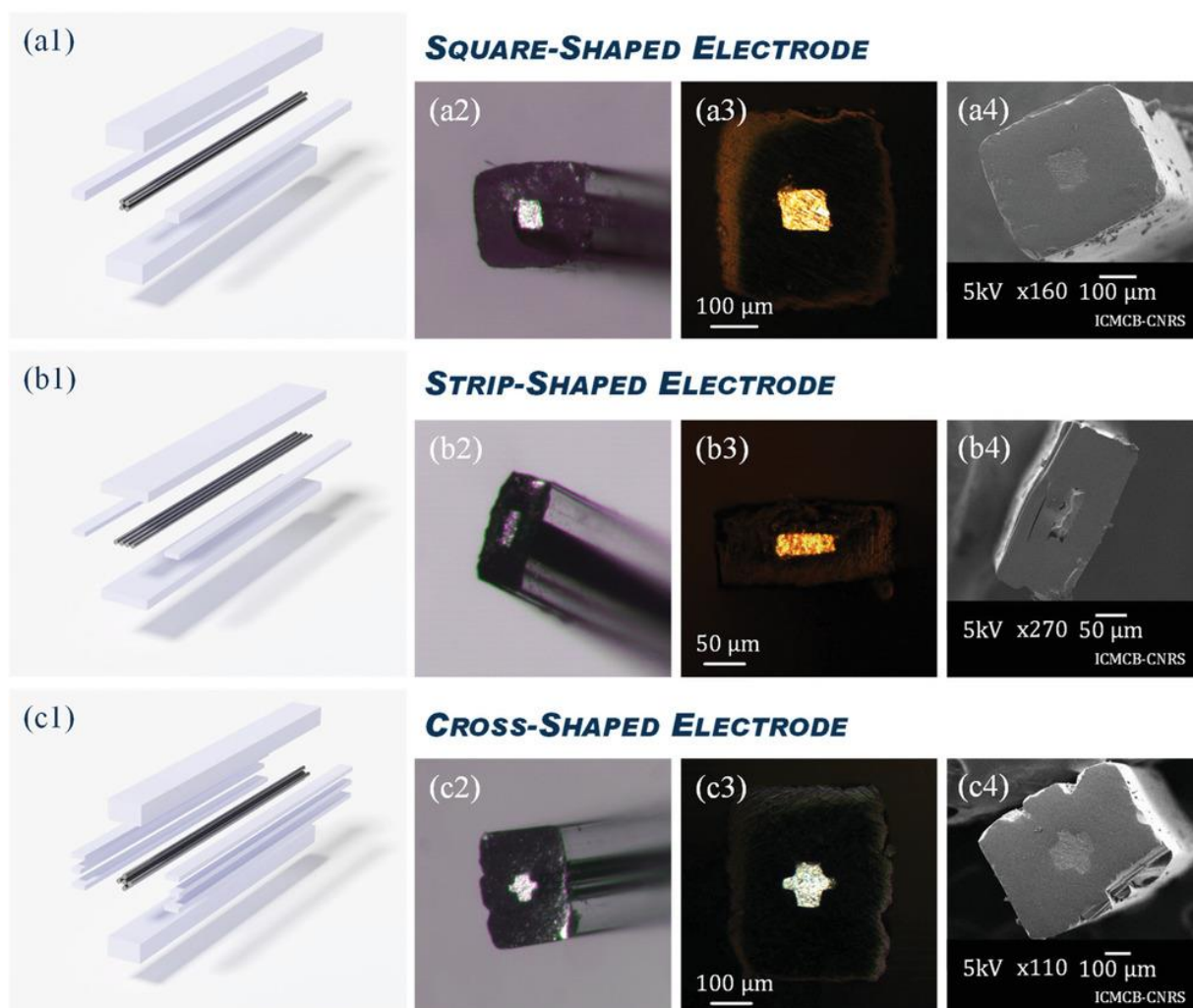
Figure 6 : a1,b1,c1) Exploded views of the preforms studied in this section. Optical microscope observations and SEM micrograph of an Al/soda–lime composite fiber with a central electrode shaped into a a1–a4) square, b1–b4) strip, and c1–c4) cross.
