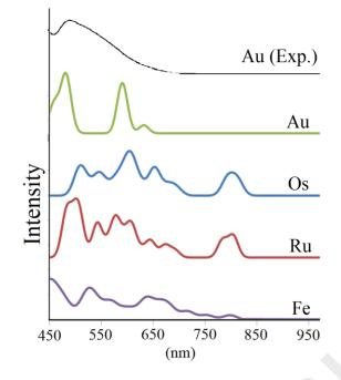
**Figure 3.** Calculated UV/Vis absorption spectra of  $[Au_{13}Cl_2(dppe)_5]^{3+}$ , and  $[M@Au_{12}Cl_2(dppe)_5]$  (M = Os, Ru, Fe). The experimental spectrum of  $[Au_{13}Cl_2(dppe)_5]^{3+64}$  is also shown for comparison.
