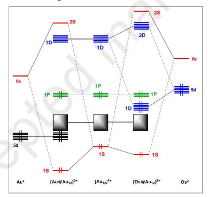
Scheme 1. Interaction of a formally  $d^{10}$  encapsulated metal atom M with an icosahedral  $[Au_{12}]^{4+}$  icosahedral cage. Left: M = gold; right: M = osmium. Note that the  $[Os@Au_{12}]^{2+}$  case is similar to that of  $[W@Au_{12}]^{.81,82}$
