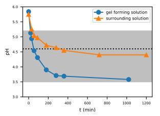
Figure 6. Evolution of pH of the surrounding solution and sample solution when not in contact with each other. The zone of pH where casein aggregation is observed is shown in gray [41]. The horizontal dotted line is the isoelectic pH.
