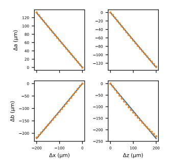
Figure 4. A typical geometric calibration of the sensor distances from the head (a, b) to the lab frame of reference (x, z)(scattered points). The error in both x and z direction are smaller than the plotted points. A linear fit (line) and matrix inversion gives the value of the calibration matrix M as  $\begin{pmatrix} -0.793 & -0.433\\ 0.736 & -0.437 \end{pmatrix}$ .
