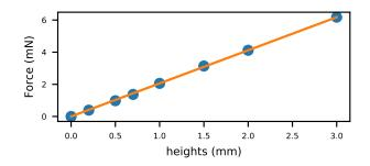
Figure 5. Cantilever stiffness calibration. The error in weight are quiet small compare to the actual measurements and hence not visible in the plot. The stiffness coefficient obtained from the linear fit is  $2.059 \pm 0.009N/m$ .
