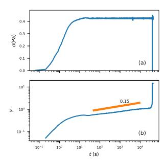
Figure 12. Constant shear stress experiment: at t = 0, the set point jumps from zero to  $\sigma = 2.13$  Pa for a gel where G' = 2.13 Pa The gap is kept constant at  $h_o = 103.8 \,\mu\text{m}$ . (a) The actually applied stress function of time. The set point is reached in 10s without overshoot. (b) The shear strain response function of time in log-log scale. The straight line highlights the power-law regime after initial convergence of the feedback loop.
