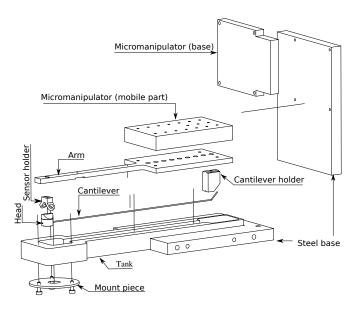
Figure 2. Exploded view of the different component of ICAMM.
