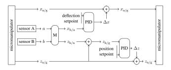
Figure 3. Diagram of the control loops in the case of a constant shear stress and a constant normal position. For the sake of space, names of reference frames are shortened to their initials.
