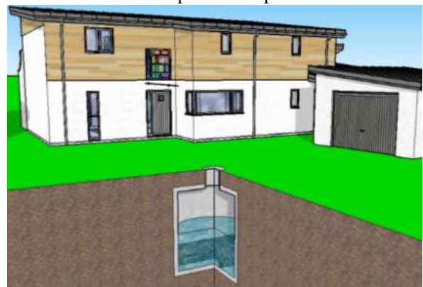
Figure 1: Example of geothermal rain water tank.
