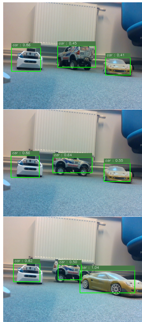
Figure 10. The object detector results deploying a pre-trained neural network model on-board the proposed scale-model vehicle prototype.
