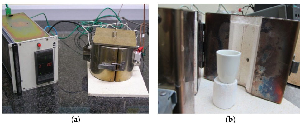
Figure 3. Setup outside (a) and oven inside (b) of the device “CIEMAT II”.
