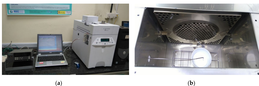
Figure 2. Setup outside (a) and oven inside (b) of the device “CIEMAT I”.
