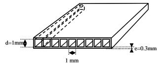
Figure 2: The cordierite dielectric geometry.
