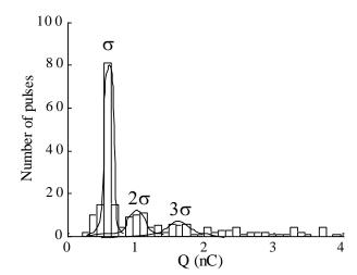
Figure 7: Corrected charge distribution in the alumina reactor.
