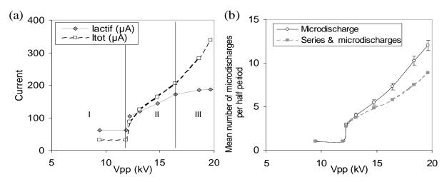
Figure 4: (a) Active and total currents (b) Number of pulses versus applied voltage for the DBD wire-to-wire.
