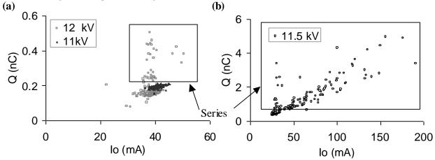
Figure 8: Representation of the pulses in the Q- $I_{\theta}$  plane for (a) wire-to-wire and (b) plane-to-plane arrangements.
