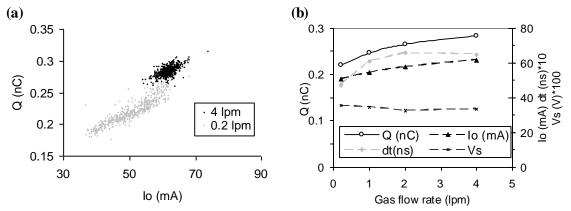
Figure 11: (a) Charge (Q) versus the maximum of the pulse current ( $I_0$ ) for each microdischarge with two gas flow rates (0.2 and 4 L min<sup>-1</sup>) (b) Evolution of the characteristics with the gas flow rate.
