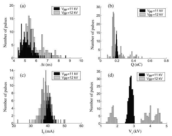
Figure 6: Distributions of the characteristics of the microdischarge in the wire-to-wire arrangement for peak to peak voltages (Vpp) of 11 and 12 kV at 60 kHz (a) Duration (b) Charge (c) Maximum current of the pulse (d) Instantaneous value of the applied voltage when the pulse occur (Vs)
