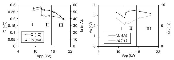
Figure 9: Evolutions of the averages characteristics with the voltage in the wire-to-wire arrangement.
