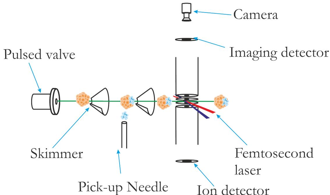
Figure 2: Experimental Setup.
