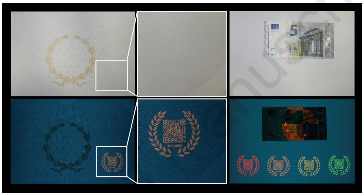
Figure 10. Top: Secured diploma from the National Institute of Applied Sciences of Rennes under day light (left) and UV irradiation ( \lambda_{\text{exc}} = 312 \text{ nm} , flux = 0.92 \text{ mW.cm}^{-2} ) (right). Bottom left: four possible security logos with color emission varying from green to red. Bottom right. Bank note under UV irradiation ( \lambda_{\text{exc}} = 312 \text{ nm} , flux = 0.92 \text{ mW.cm}^{-2} ) for brightness comparison.
