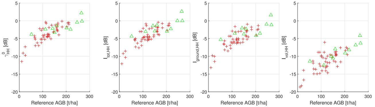
Fig. 12. SAR and tomographic HH polarized backscatter intensity as function of biomass in RE. (Left to right) SAR  $\gamma^0$ , total tomographic intensity, ground intensity ( $z = -10$  m to  $z = 10$  m) and volumetric intensity ( $z = 10$  m to  $z = 30$  m). Forest stands are marked in red while the square plots are marked in green.
