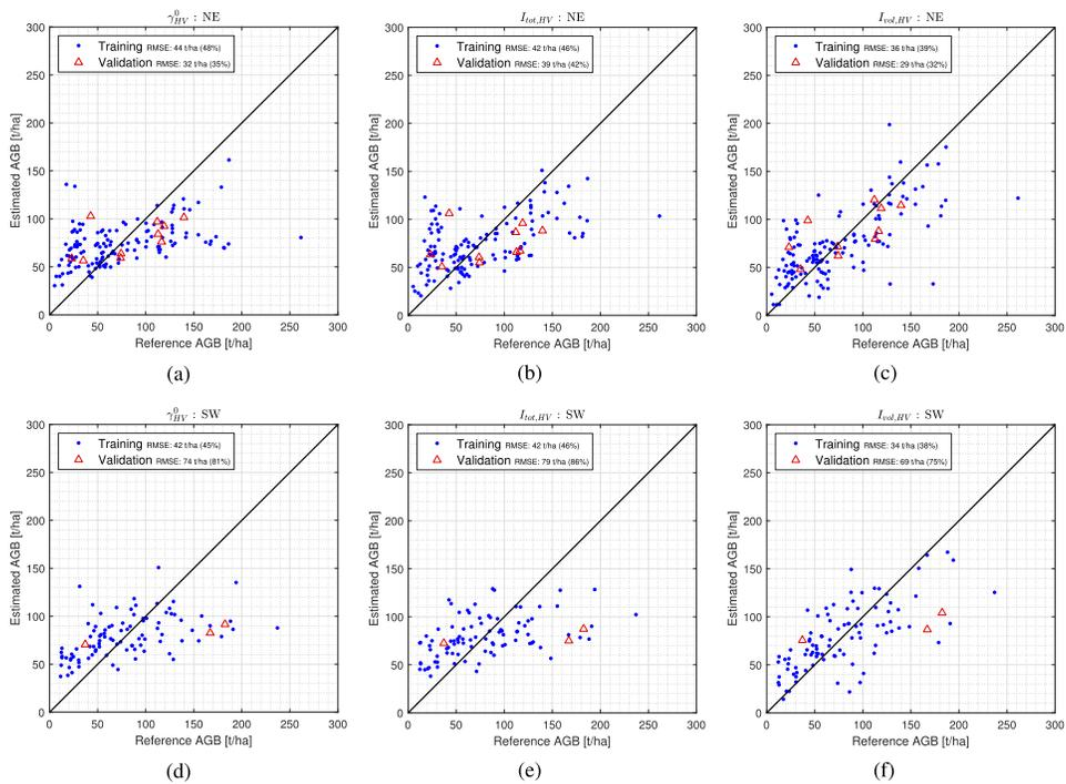
Fig. 11. SAR  $\gamma^0$  and TomoSAR  $I_{tot}$  and  $I_{vol}$  training and validation AGB retrievals for simulated BIOMASS HV polarized data. Points and triangles correspond to plots and stands shown in Fig. 3. (a) AGB retrieval using NE SAR  $\gamma^0$ . (b) AGB retrieval using NE TomoSAR  $I_{tot}$ . (c) AGB retrieval using NE TomoSAR  $I_{vol}$ . (d) AGB retrieval using SW SAR  $\gamma^0$ . (e) AGB retrieval using SW TomoSAR  $I_{tot}$ . (f) AGB retrieval using SW TomoSAR  $I_{vol}$ .
