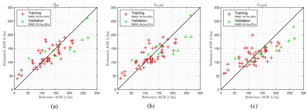
Fig. 13. AGB model training residuals obtained for the stands in RE. Forest stands are marked in red while the square plots are marked in green. (a) AGB retrieval using SAR  $\gamma^0$ . (b) AGB retrieval using TomoSAR  $I_{tot}$ . (c) AGB retrieval using TomoSAR  $I_{vol}$ .
