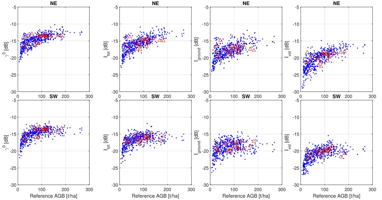
Fig. 7. SAR and TomoSAR HV polarized backscatter intensity as function of AGB for (Top) north-east looking and (Bottom) south-west looking directions. (Left to right) SAR  $\gamma^0$ , total tomographic intensity, ground intensity ( $z = -10$  m to  $z = 10$  m) and volumetric intensity ( $z = 10$  m to  $z = 30$  m). Points and triangles correspond to plots and stands shown in Fig. 3.
