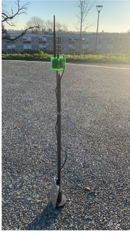
FIGURE 2 The packaged Pycom device fixed on a rod and connected to a battery
