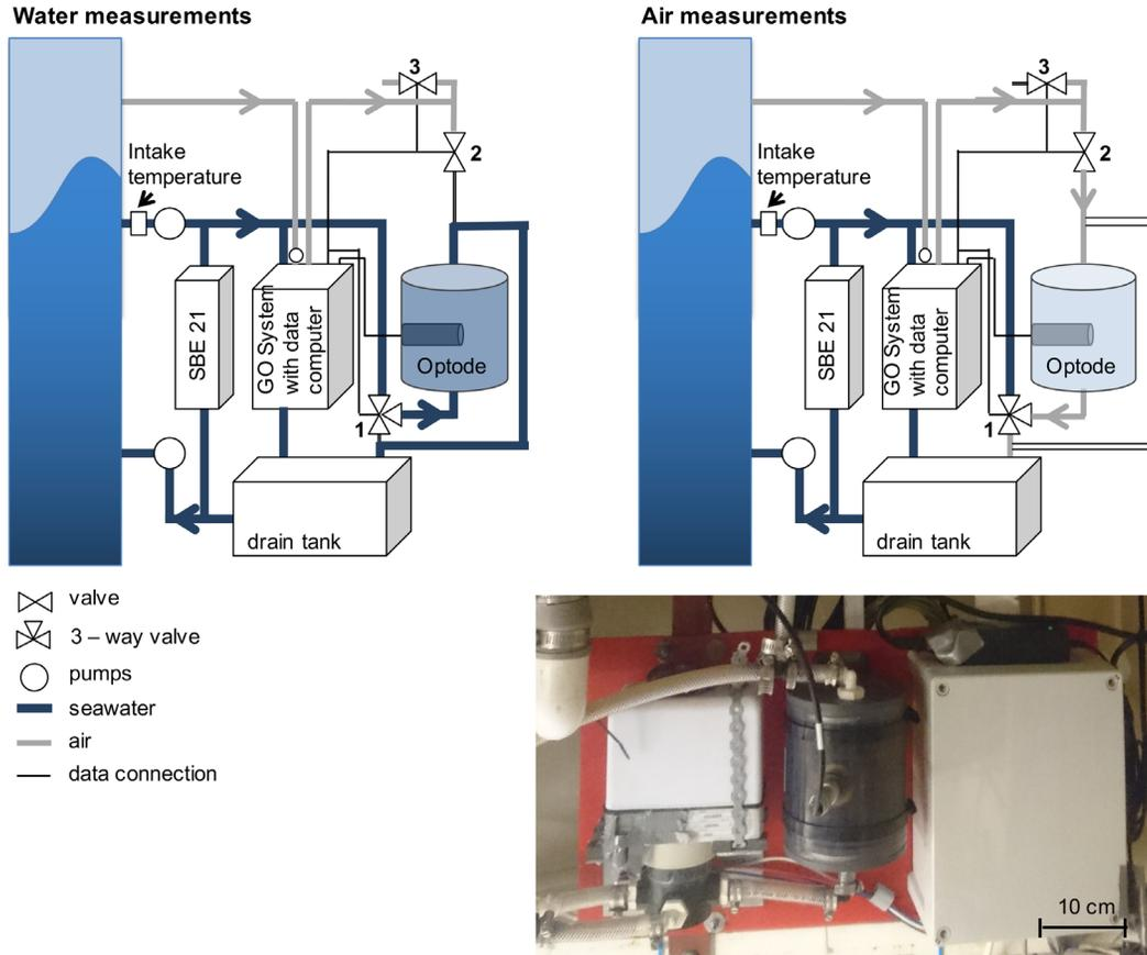
**Fig. 2.** Schematic setup of the optode in-air calibration system on Nuka Arctica during water measurements (left-hand side), during air measurements (right-hand side), and a picture of the installation.
