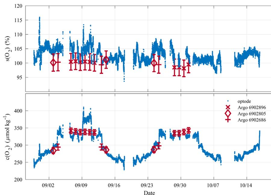
**Fig. 5.** Oxygen saturation (upper panel) and concentration (lower panel) of the underway measurements (blue) and three different Argo floats in the area (red). The error bars reflect the uncertainty of the Argo data (6902686, 6902805: 35; 6902896: 10 hPa).
