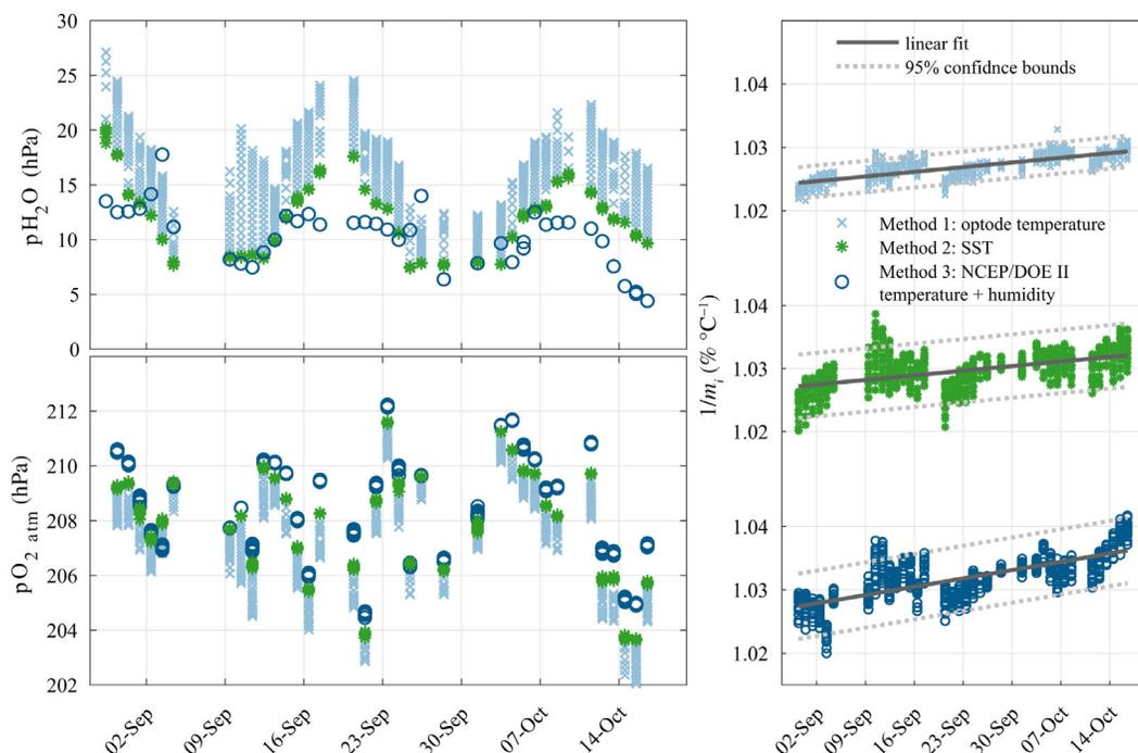
**Fig. 3.** Time series  $p\text{H}_2\text{O}$ ,  $p\text{O}_{2, \text{air}}$  and  $1/m_i$  with linear regression (dark gray lines) calculated for the three different methods (method 1: Optode temperature [light blue], method 2: SST [green], method 3: Temperature and humidity from NCEP/DOE II reanalysis [dark blue]). The 95% confidence bounds (dashed lines) of the linear regression correspond to an error of two times the standard deviation.
