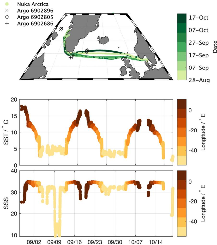
**Fig. 1.** Map showing the track of M/V Nuka Arctica and the surface temperature and salinity collected at five crossings during September/October 2018. Eastern parts are associated with warm and saline waters, while waters are colder and fresher in the west. The positions of the three Argo floats that were used for comparison are shown in black in the map.
