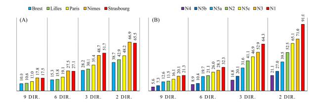
Figure 6. Mean error over the mean annual concentration compared to the reference using a regular wind direction step as a function of (A) the wind rose location and (B) the building layout (DIR: Directions).
