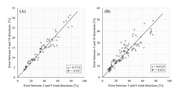
Figure 11. Estimation of the error using the first approach with regular steps when considering 6 and 9 wind directions.
