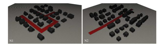
Figure 3. Illustration of the selected meshes for the N1 and N2 urban layouts (in red the roads considered as emission sources).
