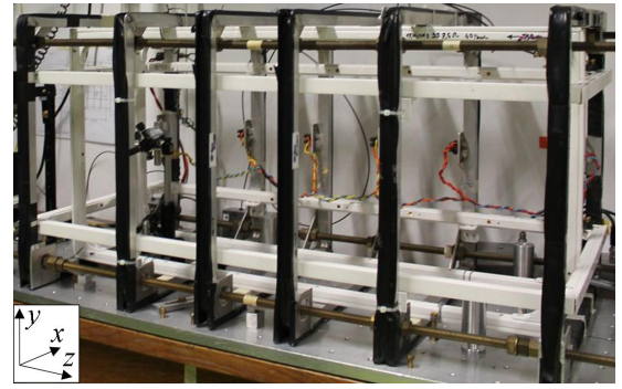
Figure 8: View of an assembled set of magnetic field coils comprising six square coils in aluminum frames (for B_z ) and two pairs of rectangular coils in white PVC wireways (for B_x and B_y ).
