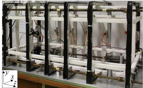
Figure 8: View of an assembled set of magnetic field coils comprising six square coils in aluminum frames (for  $B_z$ ) and two pairs of rectangular coils in white PVC wireways (for  $B_x$  and  $B_y$ ).
