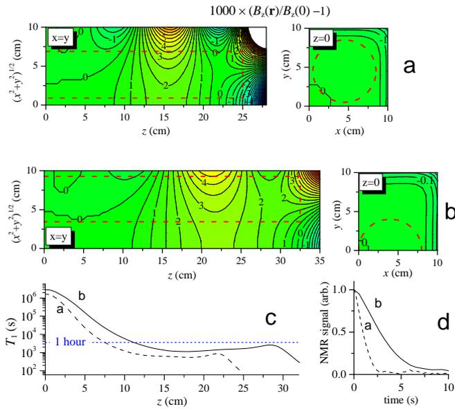
Figure 6: Computed field maps for the smaller (a) and larger (b) set of coils of Table 3, with contour lines every 0.1% (0.01% in the plane  $z = 0$  of b). The dashed lines in the maps mark the locations of  $V_{OP}$  in the diagonal planes  $x = y$  and of  $V_S$  in the planes  $z = 0$ . c: Variations of local  $T_1$  in  $V_{OP}$  for  $p = 0.4$  mbar. d: NMR signal decays in  $V_S$  at 40 kHz.
