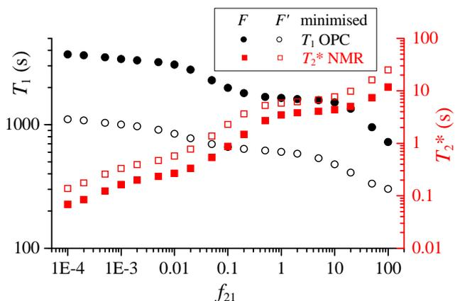
Figure 5: Computed global  $T_1$  in  $V_{OP}$  (for  $p = 0.4$  mbar) and  $T_2^*$  in  $V_S$  (for a Larmor frequency of 40 kHz, typical of actual systems) obtained for the system of Fig. 2b when minimising  $F$  or  $F'$  (see legend). The parameter  $f_{21}$  sets the relative weight of inhomogeneities in the minimisation process (Eqs. 13 and 14).
