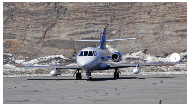
Figure 1 ONERA SAR system (SETHI) as operated in Greenland. Pod under the left wing contains the UHF antenna looking to the left at 45° incidence. Pod under the right wing contains L-band antenna looking to the left (though orientable in flight from horizon to horizon) and X-band antenna looking to the right (orientable in flight from horizon to nadir)
