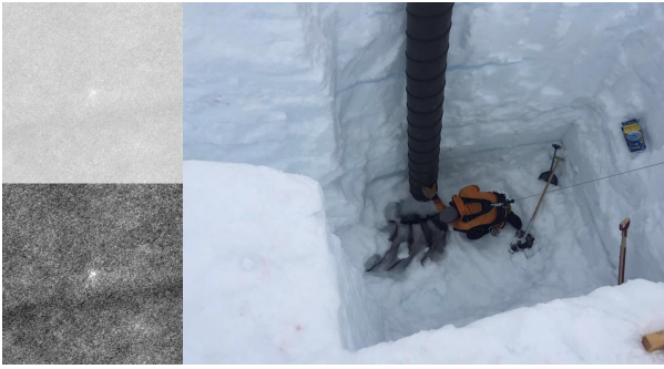
Figure 6 Candidate for fan hub fragment on the final X-band image (left). On top the genuine image and at bottom the contrast is strongly emphasised. The dark horizontal line is a crevasse under 6 m snow-bridge. Recovery of the hub fragment 15 months after radar acquisition (right). The trench is about 4 m deep, the crevasse is ahead (photographer stands on the south lip of the trench).
