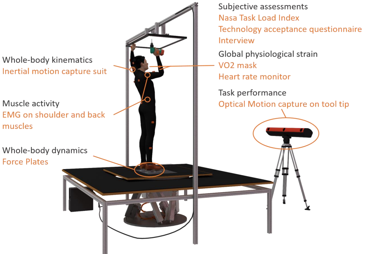
Fig. 2. Experimental set up for data recording at the laboratory experiment.
