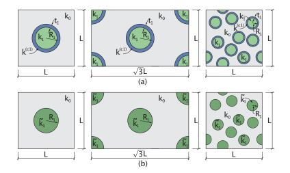
Fig 15. (a) Typical unit cell of 2D periodic three-phase composites with squarely, hexagonally and randomly distributed inclusions (three-phase model); (b) Typical unit cell of 2D periodic two-phase composites with squarely, hexagonally and randomly distributed equivalent inclusions (equivalent inclusion model)
