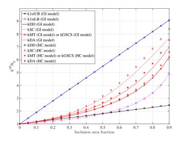
Fig9. Estimates and bounds of the normalized effective thermal conductivity, with respect to the conductivity of the matrix phase  $k_0$ , versus the inclusion area fraction of a two-phase composite with general imperfect (GI) and highly conducting (HC) interface models with  $k_1/k_0 = 10$ ,  $k^{(c1)}/k_0 = 0.1$ ,  $t_1/R_1 = 0.001$  and  $\beta_1/R_1 = t_1 k^{(c1)}/R_1 = 0.0001 k_0$ .
