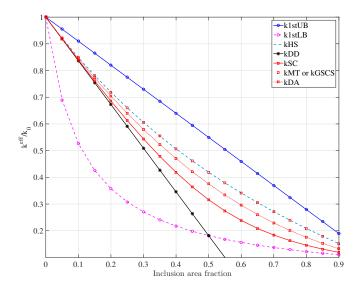
Fig6. Estimates and bounds of the normalized effective thermal conductivity, with respect to the conductivity of the matrix phase  $k_0$ , versus the inclusion area fraction of a two-phase composite with general imperfect (GI) interface model with  $k_1/k_0 = 0.1$ ,  $k^{(c1)}/k_0 = 0.5$  and  $t_1/R_1 = 0.001$ .
