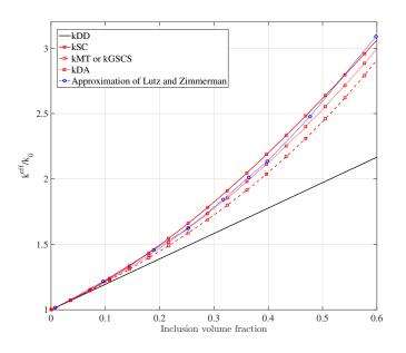
Fig 12. Estimates and comparaisons with results of Lutz and Zimmerman [40] of the normalized effective thermal conductivity, with respect to the conductivity of the matrix phase  $k_0$ , versus the inclusion volume fraction of a tridimensional two-phase composite with general imperfect (GI) interface model with  $k_1/k_0 = 10$ ,  $D = (k_0 - k_{if}^{(c1)})/k_0 = -0.75$  and  $t_1 = 2.3a_1/\rho_1 = 0.23$ .
