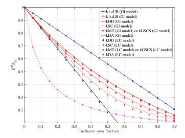
Fig 7. Estimates and bounds of the normalized effective thermal conductivity, with respect to the conductivity of the matrix phase  $k_0$ , versus the inclusion area fraction of a two-phase composite with general imperfect (GI) and lowly conducting (LC) interface models with  $k_1/k_0 = 0.1$ ,  $k^{(c1)}/k_0 = 10$ ,  $t_1/R_1 = 0.001$  and  $\alpha_1/R_1 = t_1/(k^{(c1)}R_1) = 0.0001k_0$ .
