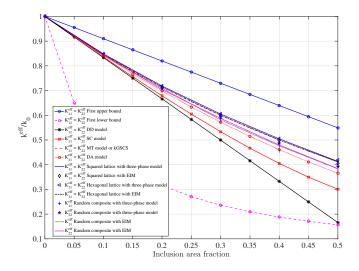
Fig17. Comparison between the effective thermal conductivities obtained by applying the EIM and three-phase model with their estimates and bounds for random and periodic composites whose  $k_1/k_0 = 0.1$ ,  $k^{(c1)}/k_0 = 0.001$  and  $t_1/R_1 = 0.001$ .
