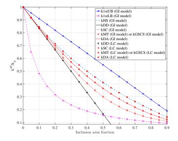
Fig8. Estimates and bounds of the normalized effective thermal conductivity, with respect to the conductivity of the matrix phase  $k_0$ , versus the inclusion area fraction of a two-phase composite with general imperfect (GI) and lowly conducting (LC) interface models with  $k_1/k_0 = 0.1$ ,  $k^{(c1)}/k_0 = 0.001$ ,  $t_1/R_1 = 0.001$  and  $\alpha_1/R_1 = t_1/(k^{(c1)}R_1) = k_0$ .
