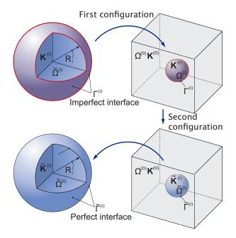
Fig4. First and second configurations used for determining the thermal conductivity tensor  $\tilde{\mathbf{K}}^{(i)}$  of the equivalent spherical inclusion  $\tilde{\Omega}^{(i)}$
