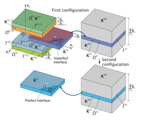
Fig2. First and second configurations used for determining the thermal conductivity tensor  $\tilde{\mathbf{K}}^{(i)}$  of the equivalent layer  $\tilde{\Omega}^{(i)}$
