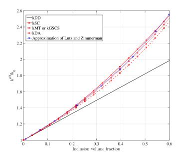
Fig 13. Estimates and comparaisons with results of Lutz and Zimmerman [40] of the normalized effective thermal conductivity, with respect to the conductivity of the matrix phase  $k_0$ , versus the inclusion volume fraction of a tridimensional two-phase composite with general imperfect (GI) interface model with  $k_1/k_0 = 10$ ,  $D = (k_0 - k_{if}^{(c1)})/k_0 = 0$  and  $t_1 = 2.3a_1/\rho_1 = 0.23$ .
