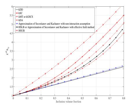
Fig14. Estimates and comparaisons with results of Sevostianov and Kachanov [41] of the normalized effective thermal conductivity, with respect to the conductivity of the matrix phase  $k_0$ , versus the inclusion volume fraction of a tridimensional two-phase composite with general imperfect (GI) interface model with  $k_1/k_0 = 10$ ,  $k_{if}^{(c1)}/k_0 = 0.7$  and  $t_1/a_1 = 0.05$ .
