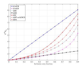
Fig5. Estimates and bounds of the normalized effective thermal conductivity, with respect to the conductivity of the matrix phase  $k_0$ , versus the inclusion area fraction of a two-phase composite with general imperfect (GI) interface model with  $k_1/k_0 = 10$ ,  $k^{(c1)}/k_0 = 5$  and  $t_1/R_1 = 0.001$ .
