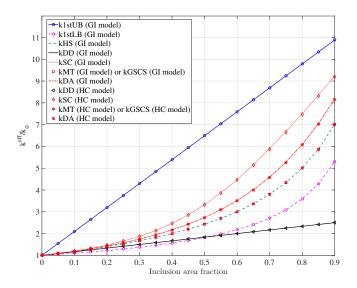
Fig10. Estimates and bounds of the normalized effective thermal conductivity, with respect to the conductivity of the matrix phase  $k_0$ , versus the inclusion area fraction of a two-phase composite with general imperfect (GI) and highly conducting (HC) interface models with  $k_1/k_0 = 10$ ,  $k^{(c1)}/k_0 = 1000$ ,  $t_1/R_1 = 0.001$  and  $\beta_1/R_1 = t_1 k^{(c1)}/R_1 = k_0$ .
