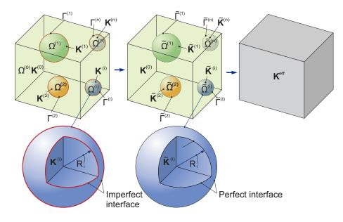
Fig 3. Two-step homogenization procedure for a spherical particle reinforced composite: (i) each spherical inclusion  $\Omega^{(i)}$  with imperfect interface  $\Gamma^{(i)}$  is replaced by an equivalent spherical inclusion  $\tilde{\Omega}^{(i)}$  with perfect interface  $\tilde{\Gamma}^{(i)}$ ; (ii) the resulting spherical particle reinforced composite is homogenized by applying classical schemes.
