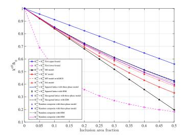
Fig16. Comparison between the effective thermal conductivities obtained by applying the EIM and three-phase model with their estimates and bounds for random and periodic composites whose  $k_1/k_0 = 0.1$ ,  $k^{(c1)}/k_0 = 10$  and  $t_1/R_1 = 0.001$ .
