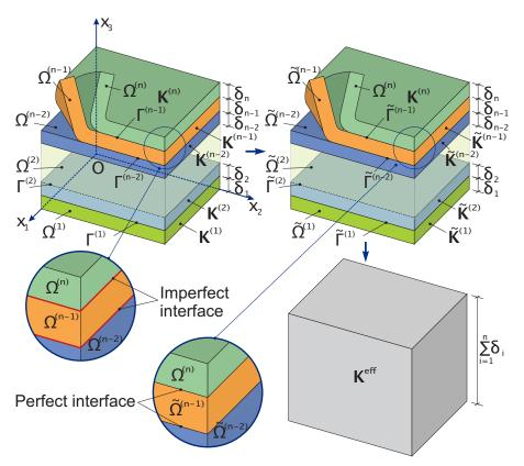
Fig 1. Two-scale homogenization procedure for a layered composite in which each layer  $\Omega^{(i)}$  with imperfect interface  $\Gamma^{(i)}$  is replaced in first with an equivalent layer  $\tilde{\Omega}^{(i)}$  with perfect interface  $\tilde{\Gamma}^{(i)}$ , then this layered composite is homogenized by applying some classical schemes.
