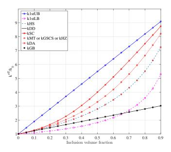
Fig 11. Estimates, bounds and comparaisons with results of Herve and Zaoui [38] and Garboczi and Bentz [39] of the normalized effective thermal conductivity, with respect to the conductivity of the matrix phase  $k_0$ , versus the inclusion volume fraction of a tridimensional two-phase composite with general imperfect (GI) interface model with  $k_1/k_0 = 10$ ,  $k^{(c1)}/k_0 = 5$  and  $t_1/R_1 = 0.001$ .
