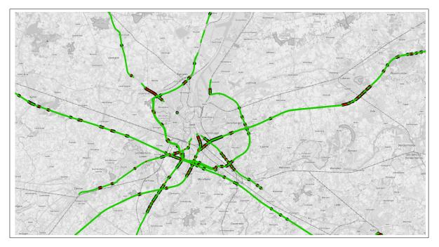
Figure 4. Accuracy of single peak pothole detector for a detection threshold of p >= 0.8. Location: Ghent, Belgium
