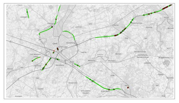
Figure 5. Accuracy of single peak pothole detector for a detection threshold of  $p \ge 0.7$ . Dataset has been reduced to only test set - meaning how would the model react to new samples?
