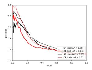
**Figure 2**. Precision - recall curves for the cases single peak detector (SP) and double peak detector (DP) with pothole labels being spread out over a radius of 2 segments. Average precision (AP) is also given.
