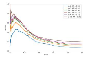
**Figure 1**. Precision - recall curves of the single peak detector. Pothole labels are spread out over neighbouring segments (*d* segments). Average precision (AP) is also given.
