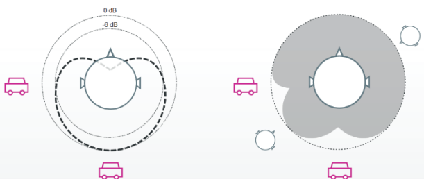
Figure 2: Left: The cardioid directivity indicates that the noise is about 6 dB louder at the back than at the side. Right: Attenuation of noise sources between speech sources [2].
