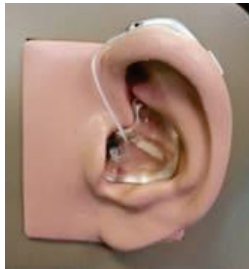
Figure 5: KEMAR artificial ear fitted with a hearing aid with a custom made earmold.
