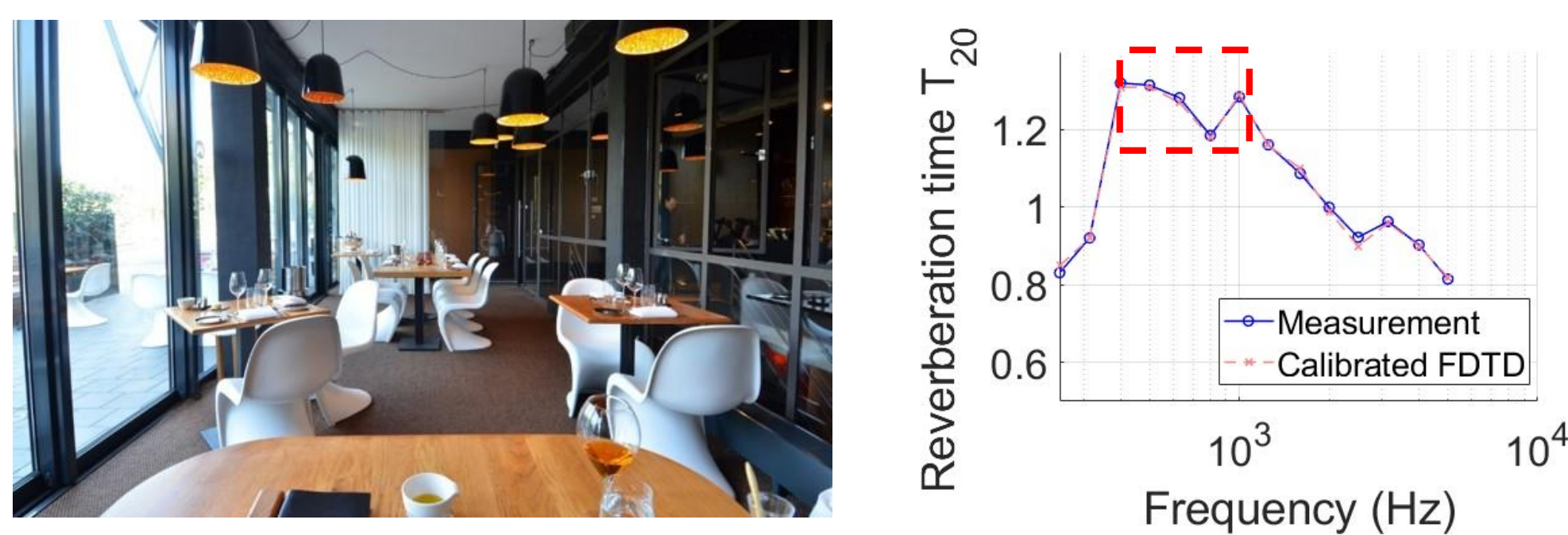
Fig. 1 Photo of the interior of the chosen space (left), T_{20} from the measurements and numerical model (right).
