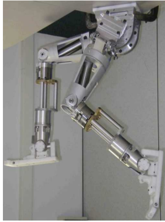
Fig. 3. Photography of the locomotor system of Hydroid .
