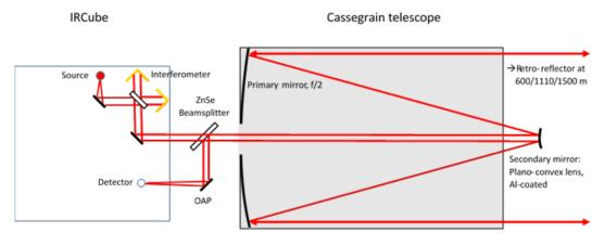
Figure 1. Schematic diagram of the setup of the OP-NIR spectrometer, its coupling to the Cassegrain telescope, and the light path through these and subsequent to/from the retroreflector.
