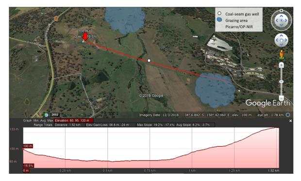
**Figure 8.** Map of the 1.55 km path at EMAI and corresponding elevation profile. The OP-NIR and stationary Picarro were located at the left end of the path and the retroreflector array at the right end. The mean elevation across the 1.55 km observation path is 118 m above sea level, an average of 23 m above surface elevation. Map © Google Earth.
