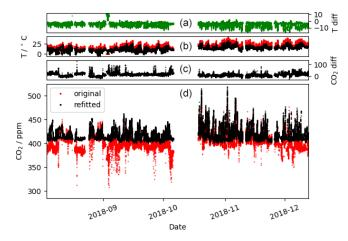
**Figure 3.** Time series illustrating the impact of re-processing the original spectra to account for contributions from short-path (spurious) reflections and inaccuracies in measured temperature. The figure shows, in order from bottom to top, the original (red) and refitted (black)  $CO_2$  (**d**), the difference between the refitted and original  $CO_2$  (**c**), the measured (red) and fitted (black) temperature (**b**), and the difference between the fitted and measured temperature (**a**).
