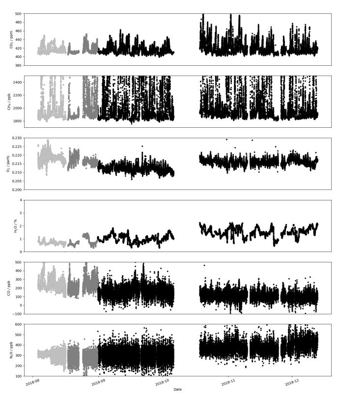
**Figure 5.** Time series of the retrieved path-averaged mole fractions for the 600, 1110 and 1500 m path lengths. Data collected at a one-way path length of 600 m are shown in light grey, at 1110 m in darker grey, and the 1500 m path length in black. The CH<sub>4</sub> y axis has been zoomed to 1700 to 2500 nmol mol<sup>-1</sup>.
