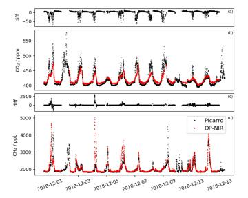
**Figure 6.** Time series of measured  $CO_2$  (**a**, **b**) and  $CH_4$  (**c**, **d**) from the OP-NIR (red) and in situ CRDS (black) measurements while the CRDS was co-located with the OP-NIR, from 1 to 13 December 2018. For each gas, the upper panel (**a**, **c**) shows the difference between the OP-NIR and CRDS measurements.
