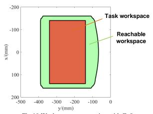
Fig.19 Workspace cross-section with Z=0
