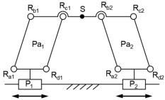
Fig.1 The diagram of 2-PPa planar parallel mechanism.
