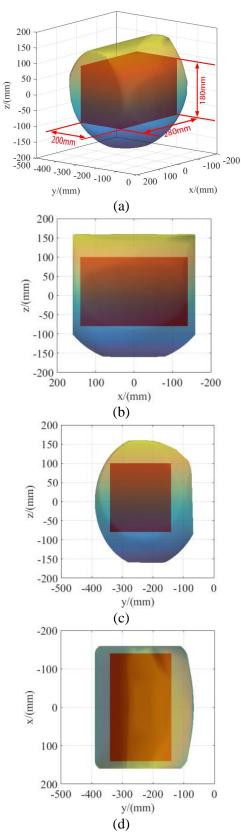
Fig.18 Task workspace inside the reachable workspace of  $SKC_2$ : (a) isometric view; (b), (c), (d) side views
