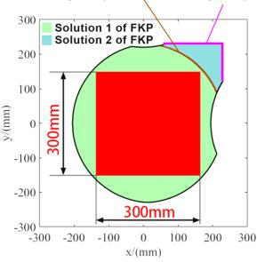
Fig.13 Workspace determined by SKC<sub>1</sub>
