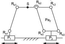
Fig.2 The alternative PRR-PPa planar parallel mechanism
