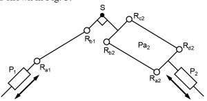
Fig.3 Modified PRR-PPa planar parallel mechanism
