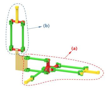
Fig.5 CAD model of Vari-Orthoglide PM
