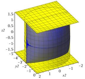
Fig.15 Serial (yellow surface) and parallel (blue surface) singularity loci of SKC<sub>2</sub>
