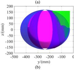
Fig.16 Workspace (pinkish) and parallel singular loci (blue) by SKC<sub>2</sub>: (a) isometric view; (b) side view normal to *X*-axis
