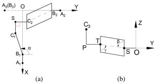
Fig.7 Side views of branch CC<sub>1</sub>: (a) projection in plane *XOY*; (b) projection in plane *YOZ*
