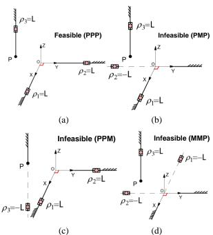
Fig.9 Feasible and non-feasible configurations: (a) PPP; (b) PMP; (c) PPM; (d) MMP
