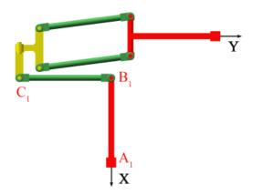
Fig. 10 Serial singularity in SKC<sub>1</sub>
