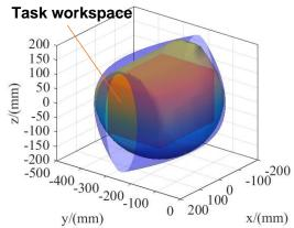
Fig.17 Singularity-free task workspace inside the reachable workspace
