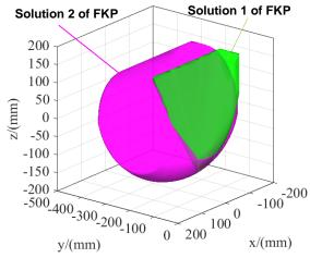
Fig.14 Maximum workspace by the SKC<sub>1</sub> and SKC<sub>2</sub>
