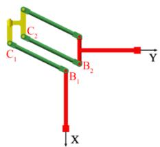
Fig.11 Parallel singularity in SKC<sub>1</sub>
