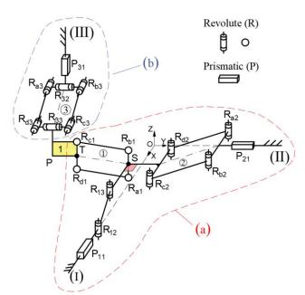
Fig.4 Schematic diagram of Vari-Orthoglide PM
