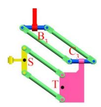
Fig.12 Parallel singularity in SKC<sub>2</sub>
