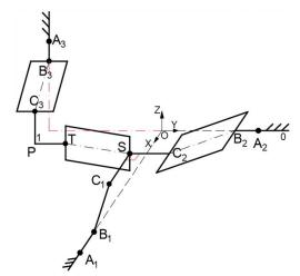
Fig.6 Simplified Vari-Orthoglide PM schematic diagram
