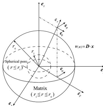
Fig. 2. The hollow sphere model.
