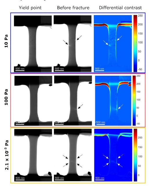
Fig. 6. Necking observations in ZrCu films deposited at 10 Pa, 100 Pa and 2.1 x 10<sup>-3</sup> Pa, from comparison of frames taken at the yield point (left) and just before fracture (middle). Subtraction of the two images (differential contrast image in the right) shows the most developed neck in the 100 Pa and 2x10<sup>-3</sup> Pa films.
