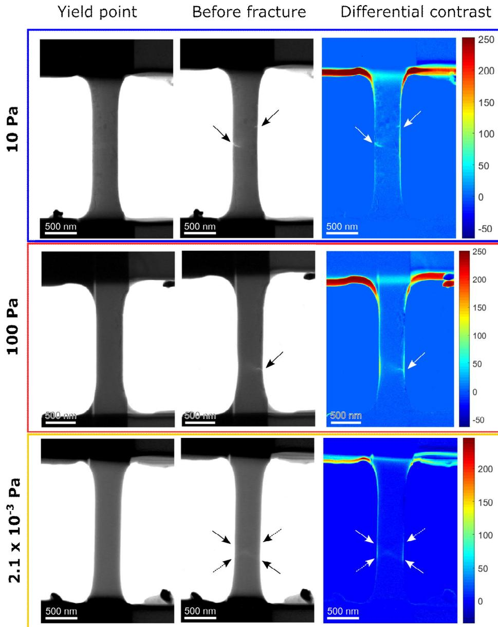
Fig. 6. Necking observations in ZrCu films deposited at 10 Pa, 100 Pa and  $2.1 \times 10^{-3}$  Pa, from comparison of frames taken at the yield point (left) and just before fracture (middle). Subtraction of the two images (differential contrast image in the right) shows the most developed neck in the 100 Pa and  $2 \times 10^{-3}$  Pa films.
