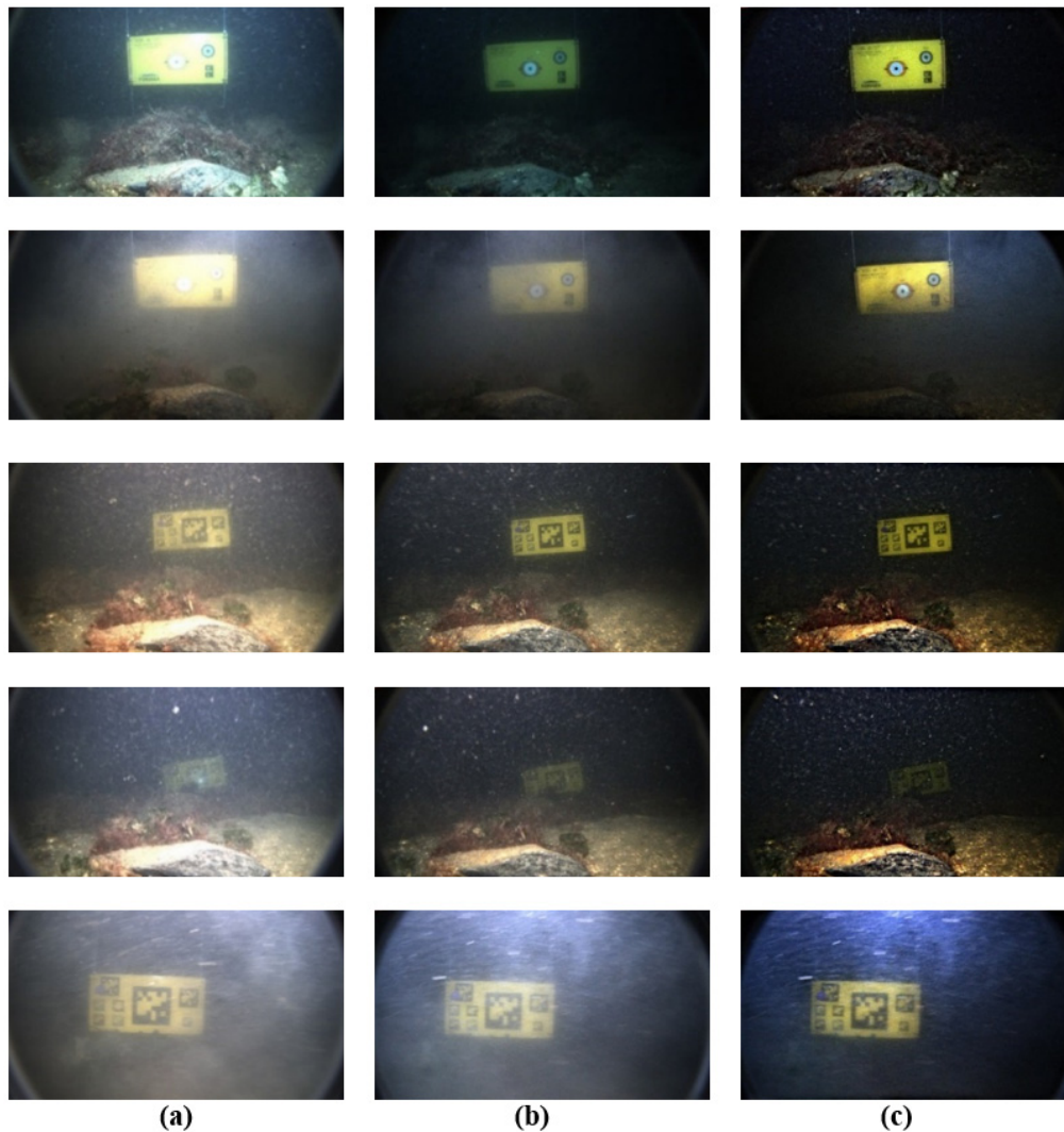
Fig. 16. Results at 8 meters deep in the port of Brest at night. (a) Images acquired without polarization, (b) images acquired with linear perpendicular-polarization, and (c) images acquired with linear perpendicular-polarization and using our processing.
