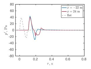
FIG. 9. (Color online) Terrain depression, C25D waves—time signals simulated at ground level at positions where the U-wave is formed, with  $\tau$  the time relative to the beginning of the waveform in the flat case.
