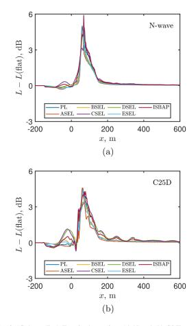
FIG. 19. (Color online) Terrain depression, (a) N and (b) C25D waves perceived noise computed at ground level using seven metrics and normalized by the flat surface case.
