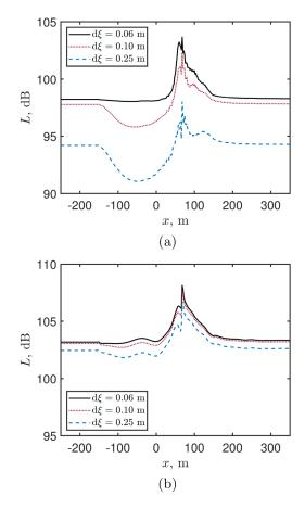
FIG. 18. (Color online) Terrain depression, N-wave—perceived noise variation along the terrain depression ground profile obtained using the (a) PL and (b) CSEL metrics with different mesh sizes.
