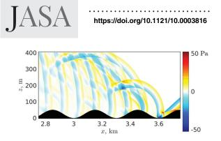
FIG. 14. Sinusoidal terrain, N-wave-pressure fluctuation map.
