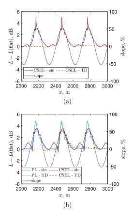
FIG. 16. (Color online) Sinusoidal terrain (sin), (a) N and (b) C25D waves—perceived noise level L computed at ground level using PL and CSEL and normalized by the flat surface case, and ground profile slope. Comparison with the isolated terrain depression (TD) case.
