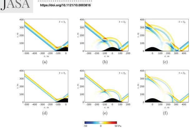
FIG. 10. Hill—pressure fluctuation maps at different instants in time  $t_1 < t_2 < t_3$  for the (top) N and (bottom) C25D waves.
