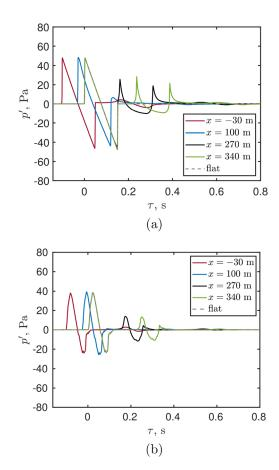
FIG. 12. (Color online) Hill, (a) N and (b) C25D waves—time signals simulated at ground level, with  $\tau$  the time relative to the beginning of the waveform in the flat case. Note the main peak at x = 340 m coincides with the flat case curve for both wave types.
