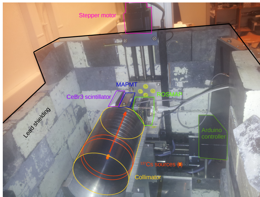
Figure 4: Photography of the automated test bench and collimated ^{137}\text{Cs} source. Source is framed in orange, collimator in yellow, \text{CeBr}_3 scintillator, MAPMT and ROSMAP electronics respectively in purple, blue and light green. The case of the arduino board is framed in dark green, and the y stepper motor in pink. The lead shielding is made of white and grey bricks and framed in black.
