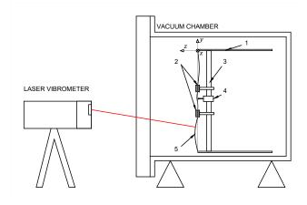
**Figure 2**: Side view: Configuration of the modal measurement, 1. Bass-drum cavity, 2. Magnets used to create null displacement boundary conditions, 3. Support structure, 4. Automatic hammer, 5. Membrane.
