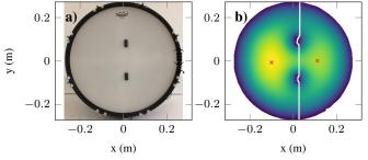
**Figure 3**: a) Frontal view of the membrane with the fixed points on the surface. b) Measurement of the landscape function by q quasi-static measurement. The red crosses mark the peak values in each sub-region.
