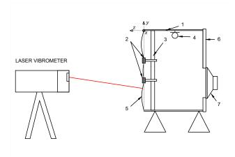
**Figure 1**: Side view: Configuration of the landscape measurement, 1. Bass-drum cavity, 2. Magnets used to create null displacement boundary conditions, 3. Support structure, 4. Microphone, 5. Membrane, 6. Back enclosure, 7. Loudspeaker.
