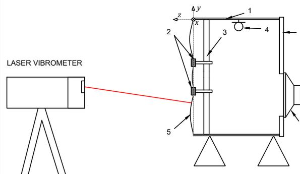
**Figure 1:** Side view: Configuration of the landscape measurement, 1. Bass-drum cavity, 2. Magnets used to create null displacement boundary conditions, 3. Support structure, 4. Microphone, 5. Membrane, 6. Back enclosure, 7. Loudspeaker.
