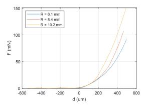
**Figure 2**. Force as function of displacement for 3 half spheres of different radius.
