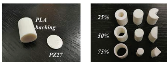
Figure 7. Transducer components. (a) piezoceramic disc PZ27 and intact PLA backing; (b) nine 3D printed PLA backings.
