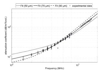
Figure 3. Attenuation coefficient due to clay powder
