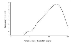
Figure 1. Particles size distribution of clay powder
