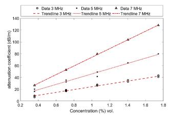
Figure 2. Attenuation coefficient due to clay powder.
