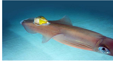
Figure 4. Squid with data-logging tag, called ITAG, attached to the dorsal surface of the squid rostrum, and positioned in line with the squid body to reduce drag (Mooney et al., 2015).
