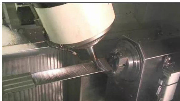
Fig. 4. Machining process of the turbine blades
