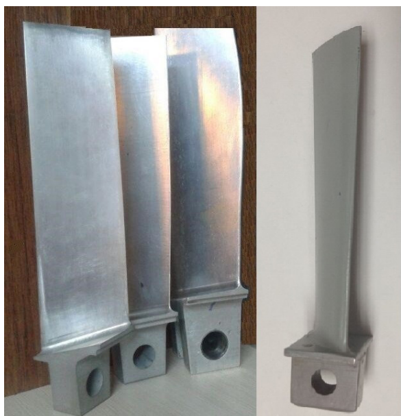
Fig. 5. The real machined turbine blades
