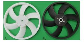
**Figure 1.** Photographies of (a) a rotational moulded fan and (b) the reference aluminium machined fan
