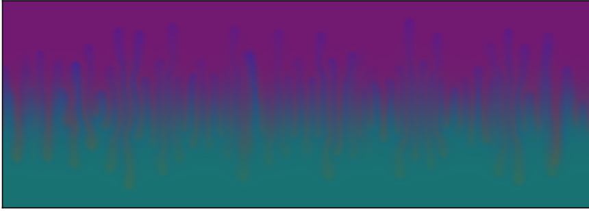
FIG. 10. Snapshot of the viscous fingering induced by reverse diffusion at t^* = 3 . A portion of the whole domain ( x = 4100\text{--}4800 , y = 0\text{--}2000 ) is plotted using the same aspect ratio for both x and y axes. The plot is rotated by 90^\circ . The invading fluid is flowing from the bottom to the top of the figure.
