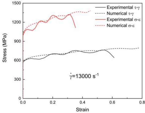
Fig. 15. Comparison of flow stress curves between experiments and numerical simulations by the MJC model at strain rate of 13000 s<sup>-1</sup>.
