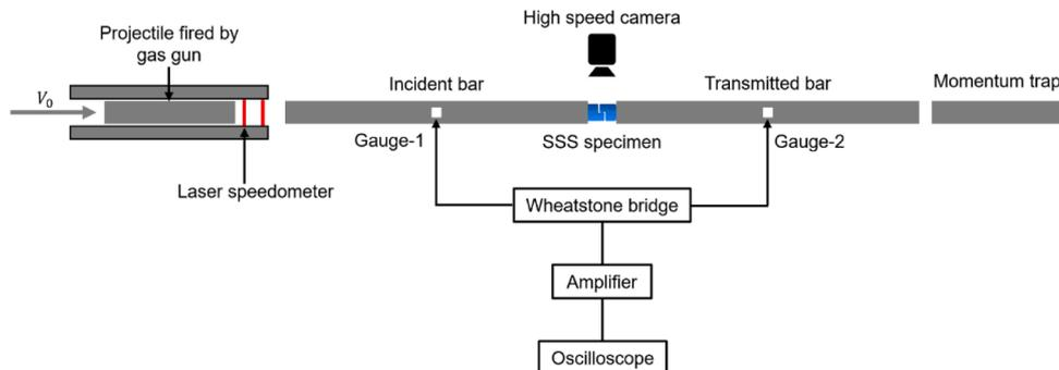
Fig. 3. Schematic presentation of the classical SHPB apparatus.
