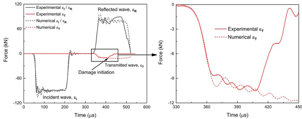
Fig. 14. Comparison of force wave signals between experiments and numerical simulations by the MJC model at strain rate of 13000 s<sup>-1</sup>.
