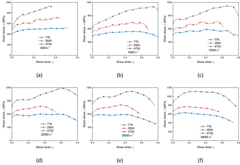
Fig. 7. Shear stress-shear strain curves at indicated temperatures under dynamic strain rates: (a)  $3000 \text{ s}^{-1}$ , (b)  $6000 \text{ s}^{-1}$ , (c)  $13000 \text{ s}^{-1}$ , (d)  $22000 \text{ s}^{-1}$ , (e)  $26000 \text{ s}^{-1}$  and (f)  $39000 \text{ s}^{-1}$ .
