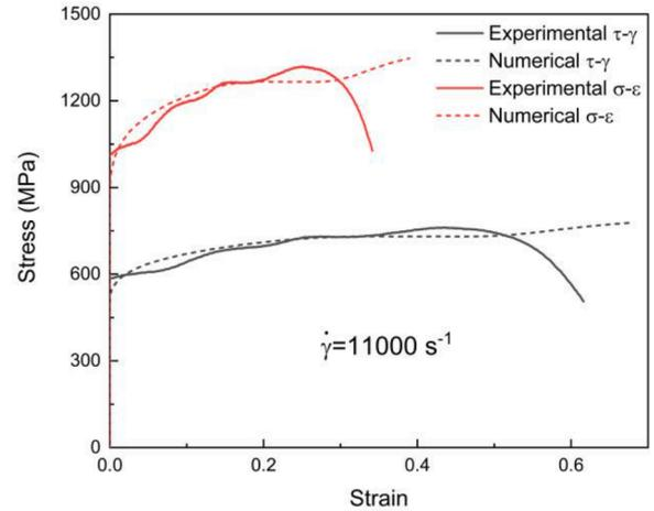
Fig. 16. Comparison of flow stress curves between experiments and numerical simulations by the MJC model at strain rate of 11000 s<sup>-1</sup>.
