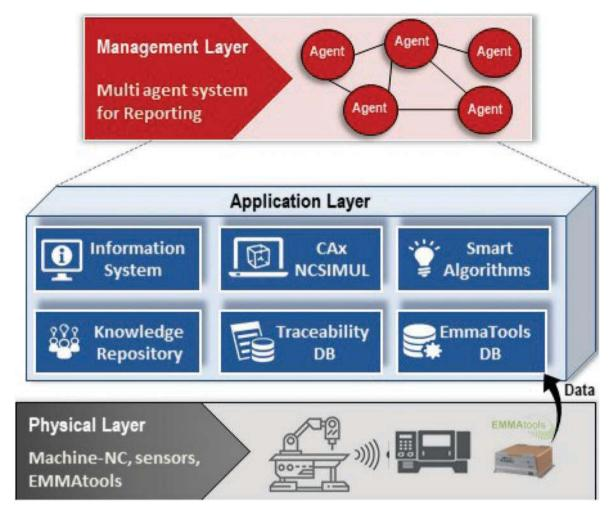
Figure 2. The Conceptual architecture.
